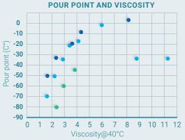
Lower the pour point, lower the temperature at which the fluid still flows.
