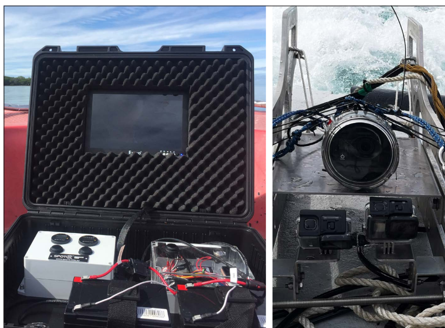
Plate 3.3 Topside video viewing console and towed underwater camera
