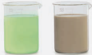
Comparison of Folia's appearance with that of a soluble oil after machining.
