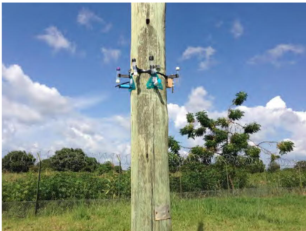
Figure 1. Palmes Diffusion tube and Radiello samplers monitoring ambient air quality at AQ3.
