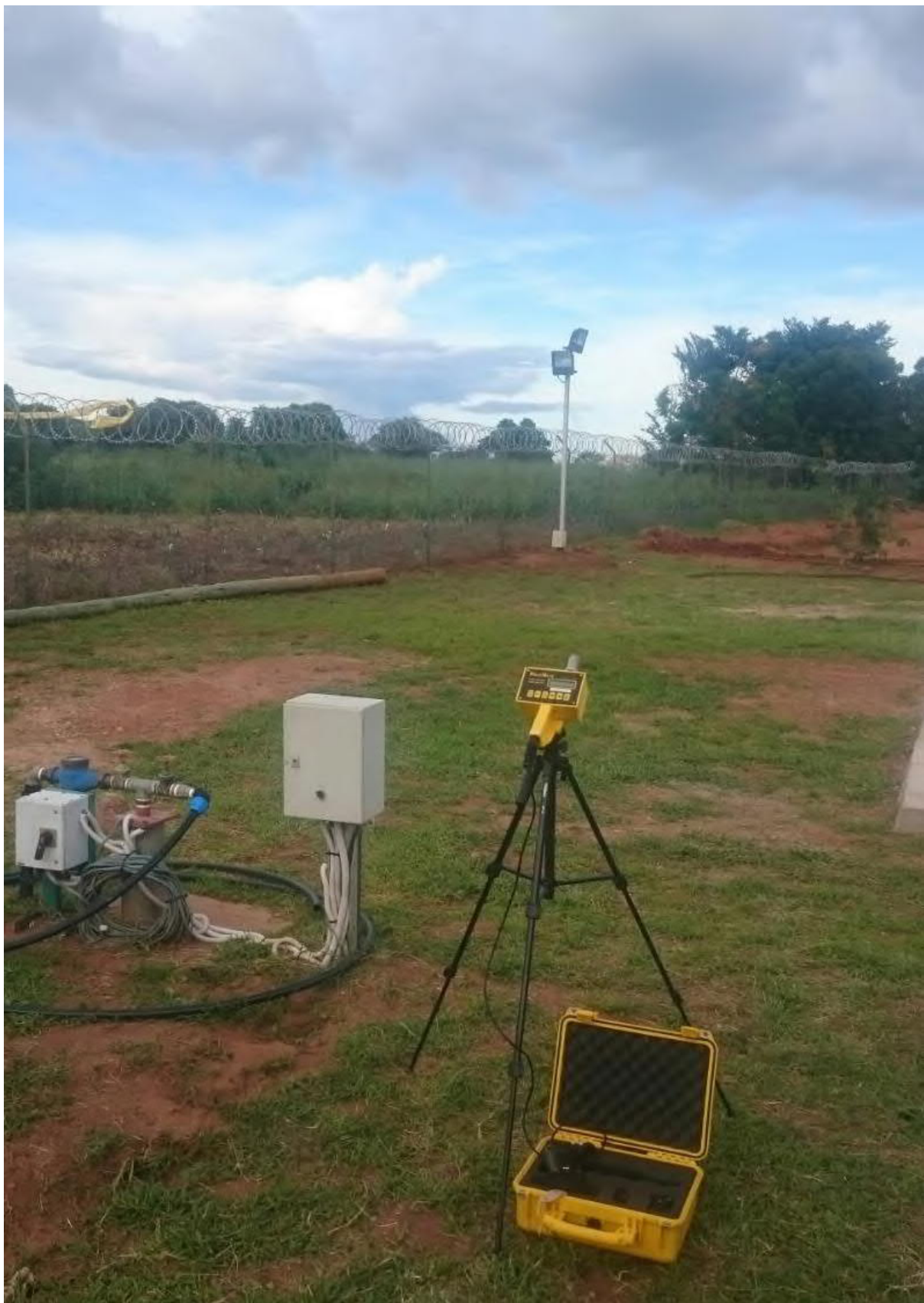
Figure 2. DustMate monitoring ambient air quality at AQ3A
