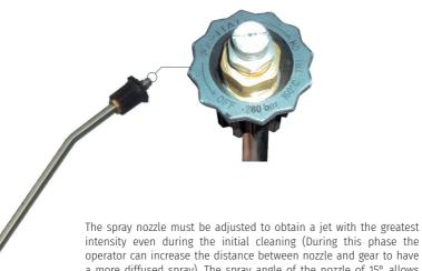
intensity even during the initial cleaning (During this phase the operator can increase the distance between nozzle and gear to have a more diffused spray). The spray angle of the nozzle of 15° allows a perfect concentration of the jet of LUBRICLEAN EP on the working flanks during cleaning.
