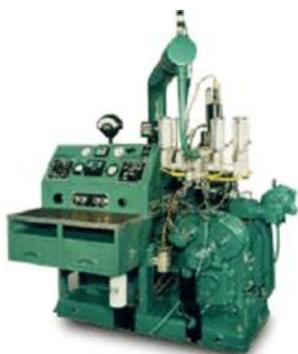
CFR diesel engine
