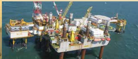
At first, the L7-CC central complex consisted of three platforms. A well platform, accommodation platform and production platform.
