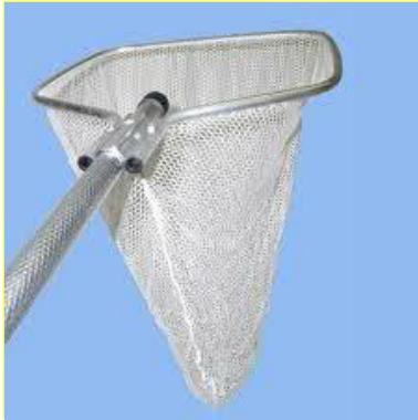
Figure 7: An example of a dip net for sampling aquatic herpetofauna and tadpoles
