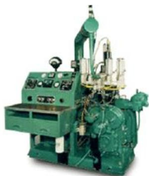
CFR diesel engine
