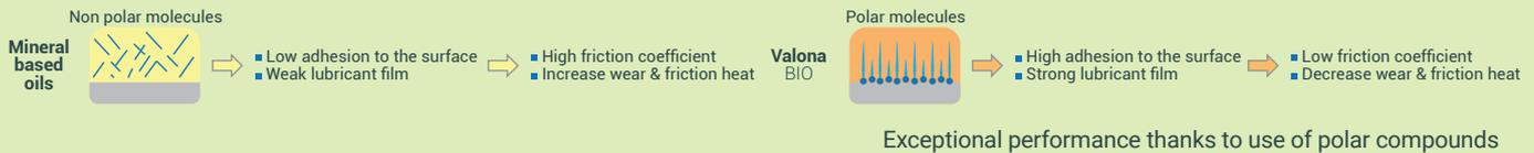
Valona BIO can be used in Minimum Quantity Lubrication (MQL) systems.
