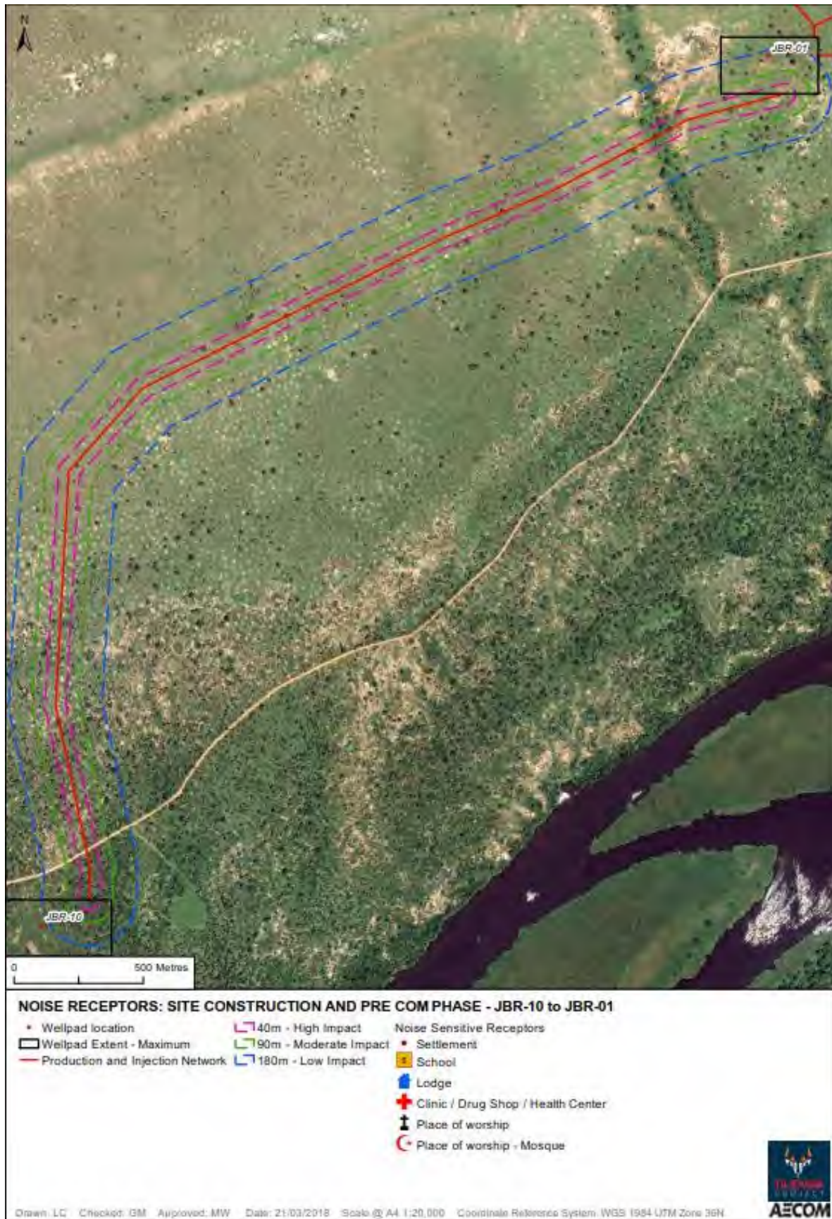
Figure I3-50: Production and Injection Network Construction Receptor Analysis – JBR-10 to JBR-01
