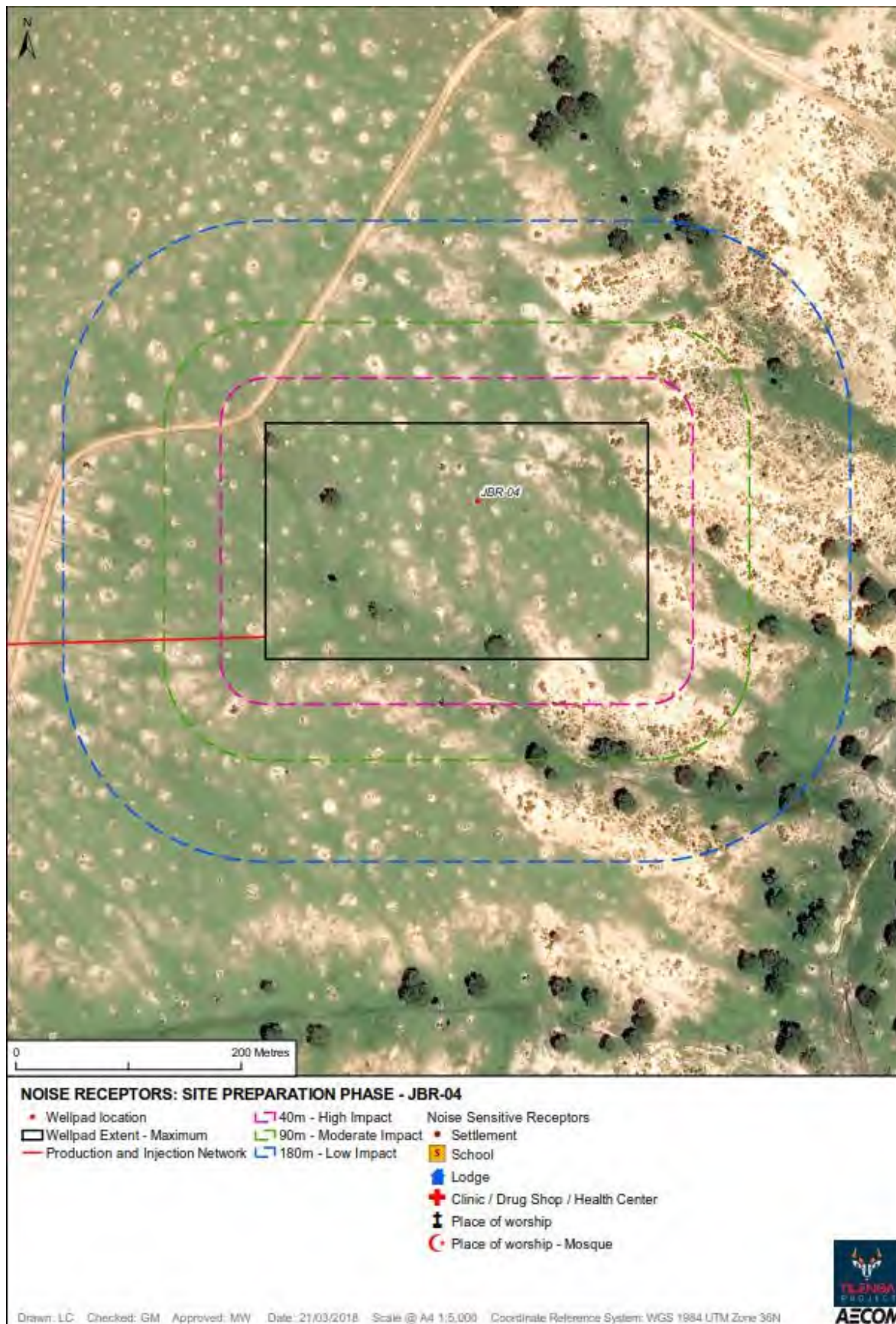
Figure I2-11: JBR-04 Site Preparation and Enabling Works Daytime Receptor Analysis
