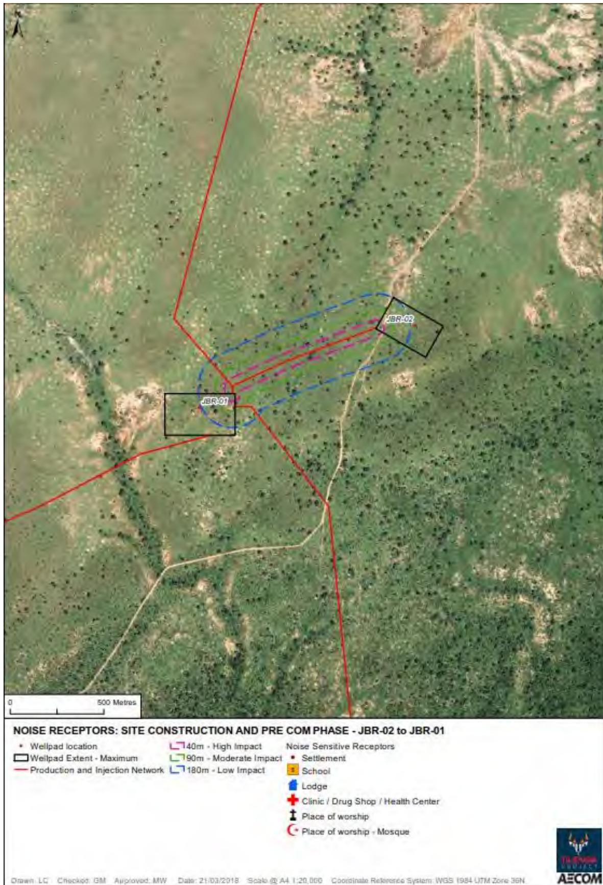
Figure I3-42: Production and Injection Network Construction Receptor Analysis – JBR-02 to JBR-01
