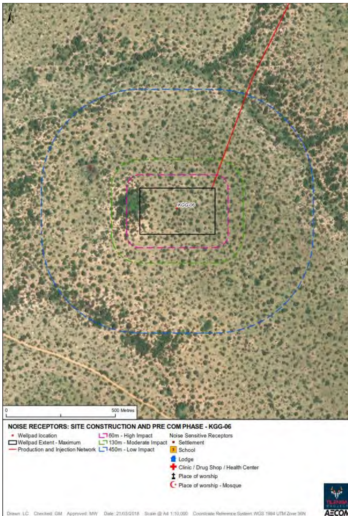
Figure I3-20: KGG-06 Night-time Well Pad Drilling Receptor Analysis
