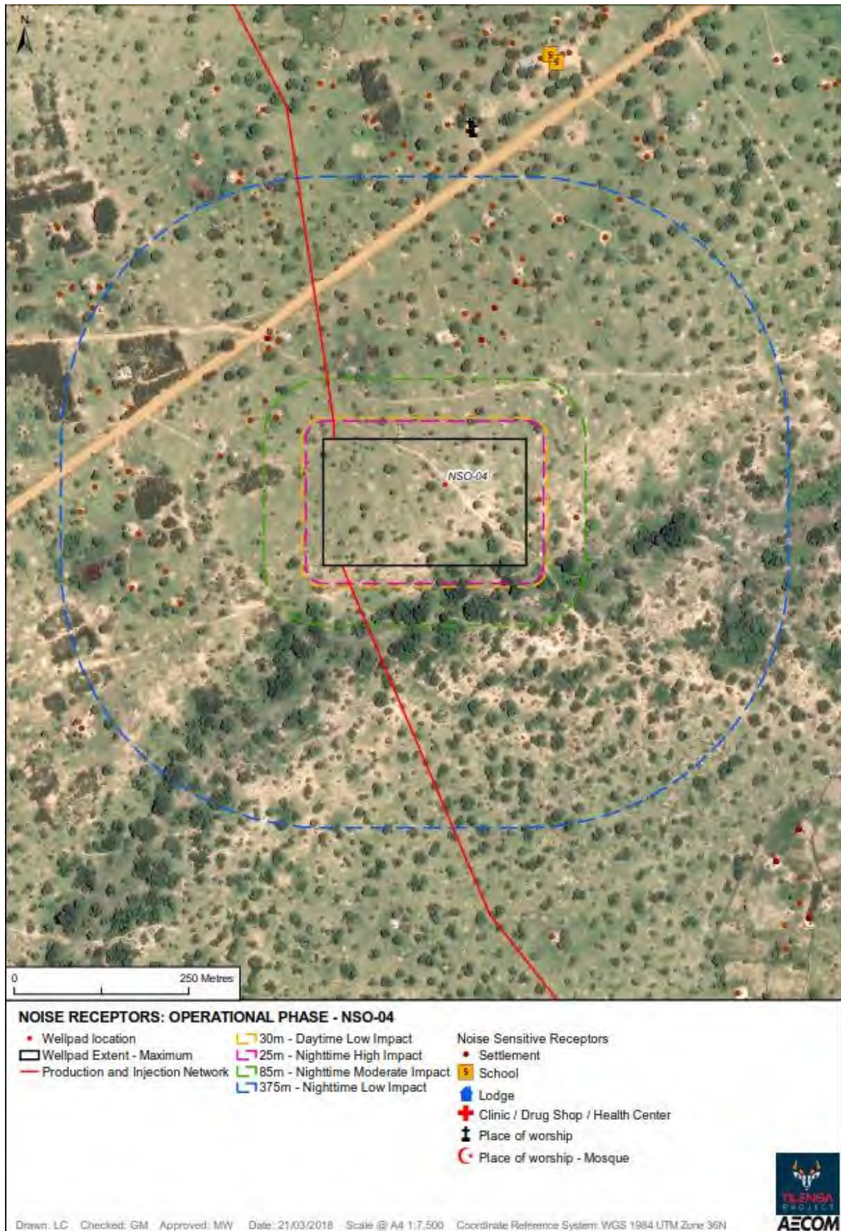
Figure I4-36: NSO-04 Commissioning and Operation Receptor Analysis
