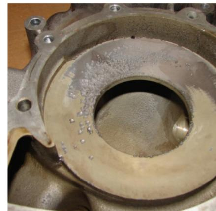
Cavitation in a waterpump (heavy duty application)
