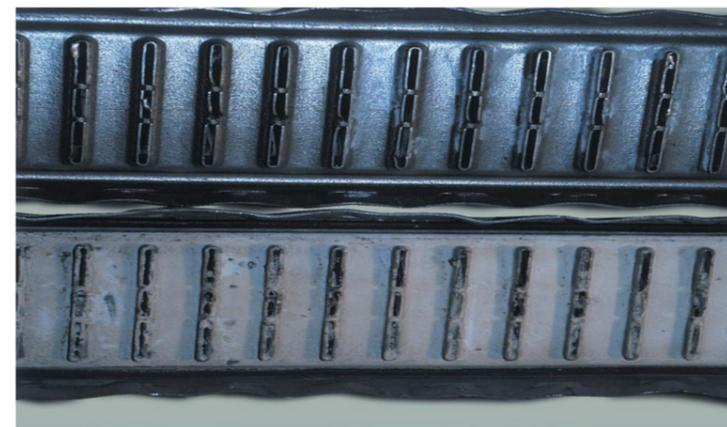
Deposit scaling on a radiator
