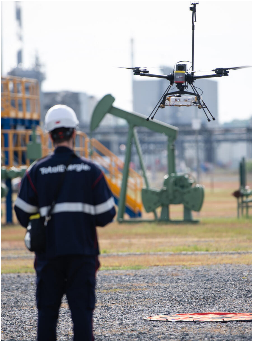
TotalEnergies uses AUSEA technology to detect and reduce methane and CO2 emissions at our sites.
