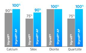
Passive adhesion test EN 15626
