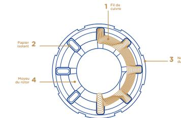
The fluid and new components of the electric vehicle are in direct contact. New challenges must be faced in terms of the fluid being compatible with different types of materials in order to avoid swelling, breakage, corrosion etc. Copper is a key material for these applications.
