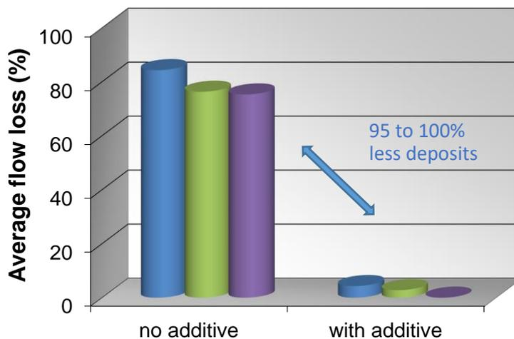
Excellium Pro Concentrate almost totally prevents injector deposits build-up with premium type of performance (<5% flow loss). The additive has been tested with various origins of regular diesel fuel.
