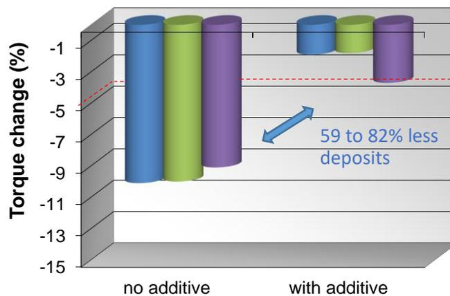
**Excellium Pro Concentrate** almost totally prevents injector deposits build-up with premium type of performance and in this manner protects the engine of torque losses (the test is considered as a clear pass when torque change is above -4,7%). It ensures stable engine power and long-term efficiency. The additive has been tested with various origins of regular diesel fuel.
