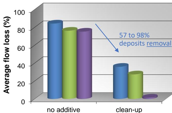
In-line with the previous keep-clean results, **Excellium Pro Concentrate** reduces existing injectors deposits. Depending on the base fuel type, this reduction ranges from half (minimum) to almost total reduction.
