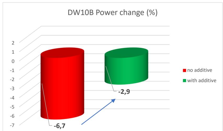
The results show that fuel treated with **Excellium Pro Concentrate** allows to recover almost 60% of power loss experienced during initial dirty-up in just one test. This is an indication of progressive removal of deposit build-up which has happened during the dirty-up phase.
