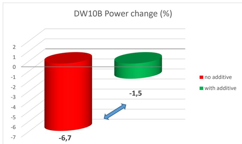
The results show that fuel treated with **Excellium Pro Concentrate** protects the engine regarding power loss (being superior to -2%, it is considered as a clear pass) as opposed to untreated fuel.
