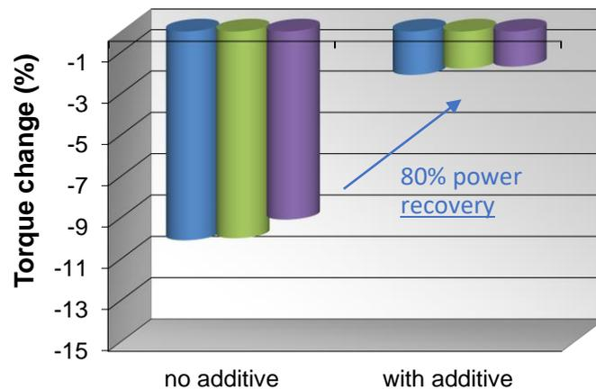
In-line with the previous keep-clean results, **Excellium Pro Concentrate** reduces significantly existing injectors deposits (this happens when torque loss after clean-up is better than after dirty-up by more than 2.5%) and allows to get back almost to the initial performance of the engine. The additive has been tested with various origins of regular diesel fuel.
