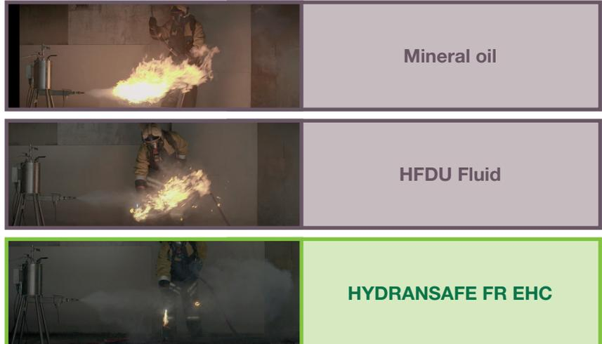
**Spray Ignition Test (DIN ISO 15029-1)** : In this test, a fire source is applied on an oil spray.
