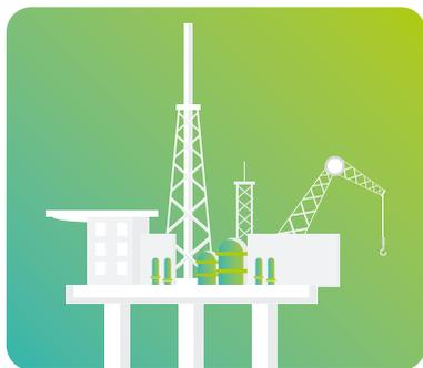
On the platform, there will be a compressor that injects the CO<sub>2</sub> into the reservoir. With only a few modifications, an existing platform can be used for carbon storage. It is also possible to construct a completely new compressor station.
