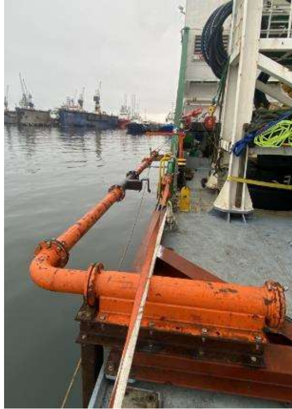
Figure 43. BSL USBL pole installation
