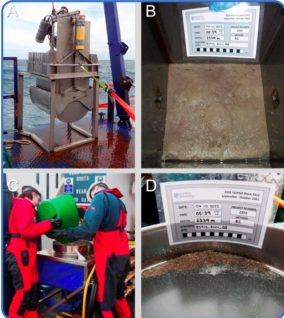
A: Grey O'Hara box corer B: largely consisted of soft pale mud over consolidated clay C: Wilson Autosiever (WAS) D: 500 \mu m sieve
