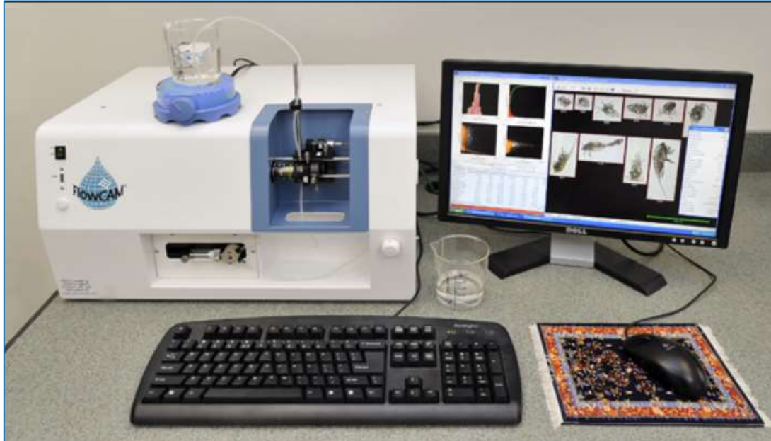
Figure 51. FlowCAM technology used to measure/count and classify organisms between 20 µm and 200 µm
